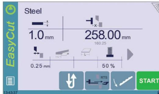
The EasyCut page is used for individual cuts, for example when an external worker needs to interrupt production just to make a single cut.
